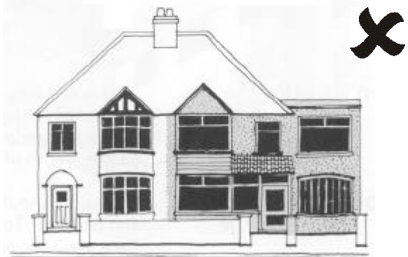
Unsatisfactory flat roof and unsympathetic materials
